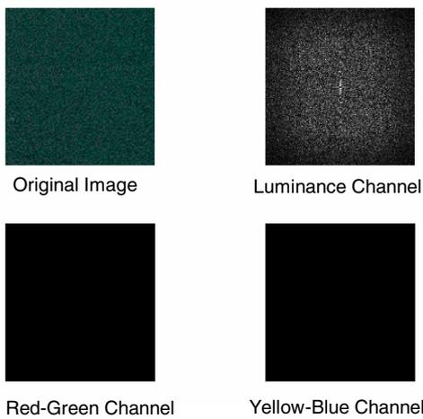
Figure 2. An original image of a metallic paint panel (top left) and its Fourier spectrum images for luminance (top right) and chromatic channels: red-green channel (bottom left) and yellow-blue channel (bottom right). Note that the DC component is in the centre of each Fourier spectrum image and that spatial frequency increase from the centre to outwards.
