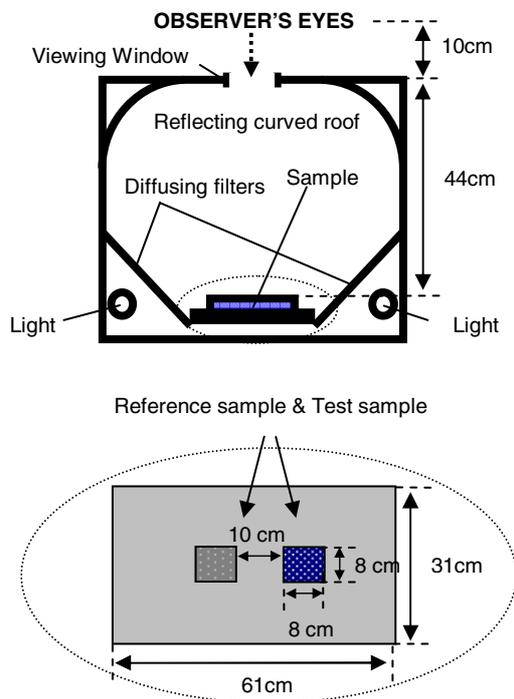
Figure 1. Schematic diagram of a DigiEye® Viewing Cabinet (top). Samples are placed on the base. Two light sources are positioned at the 2 bottom corners at each side and both emit light to the walls. The top corners have curved surfaces to reflect light uniformly onto the sample. An observer looked down the sample from the viewing window. An illustration of samples' arrangement and an observer's viewing field (bottom).
