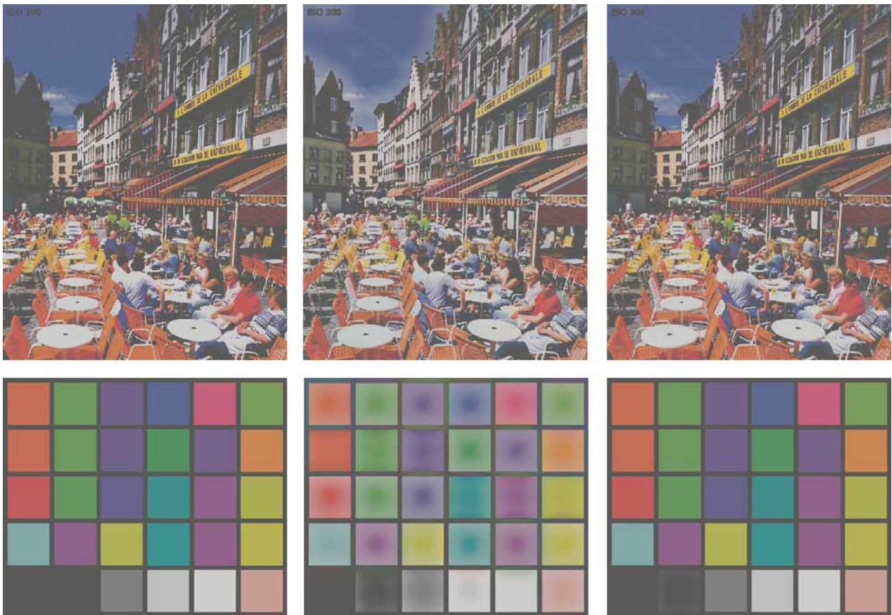
Figure 5. Effect of edge preserving smoothing to avoid halos: mapped image I_M (left), image I_{EM} using conventional unsharp masking (middle), I_{EM} using edge preserving smoothing
