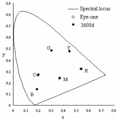
**Figure 2.** Comparison of chromaticity coordinates resulted by the two spectrometers for red(R), green(G), blue(B), cyan(C), magenta(M) and yellow(Y) chips of ColorChecker.
