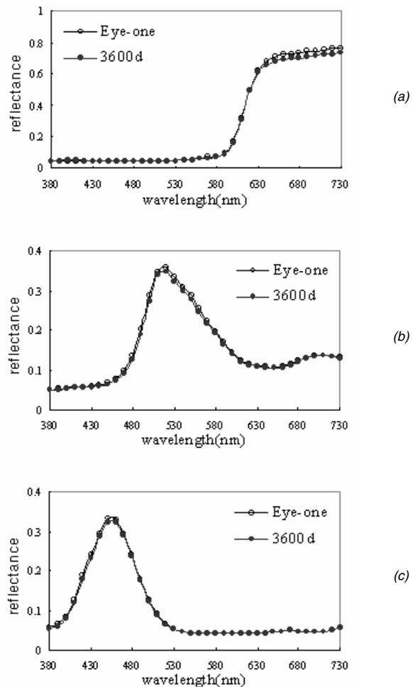
Figure 1. Comparison of reflectance measured by Eye-one and 3600d spectrometer for (a) red, (b) green and (c) blue chips of ColorChecker.
