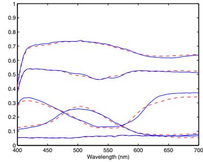
**Figure 1.** Good spectral estimation - training set: Munsell 200/II, camera: Fuji. Solid line: original spectra, dashed line: estimated spectra.
