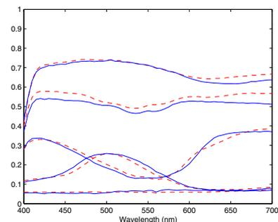
**Figure 3.** Good spectral estimation - training set: Munsell 200/II, camera: Canon. Solid line: original spectra, dashed line: estimated spectra.
