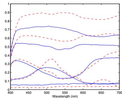
**Figure 2.** Bad spectral estimation - training set: Macbeth, camera: Fuji. Solid line: original spectra, dashed line: estimated spectra.
