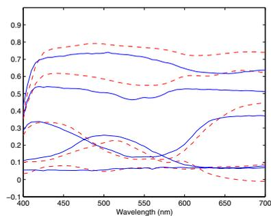
**Figure 4.** Bad spectral estimation - training set: Macbeth, camera: Canon. Solid line: original spectra, dashed line: estimated spectra.
