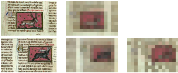
Figure 2. Two images (left) and the associated thumbnails (middle), made of n = 10 \times 15 pixels. Each pixel of a thumbnail is associated to a feature in 5 dimensions (L, a, b, X, Y) . All of them have the same weight. In this context, EMD is equivalent to an assignment problem. Each pixel of the query image (top left) is assigned to exactly one pixel of the target image. To illustrate the EMD operation, the thumbnail on the right represents the optimal permutation of the query pixels to match the target. The query pixels of the red region are moved towards their location in the target image. The white column of paper is also correctly moved from right to left.
