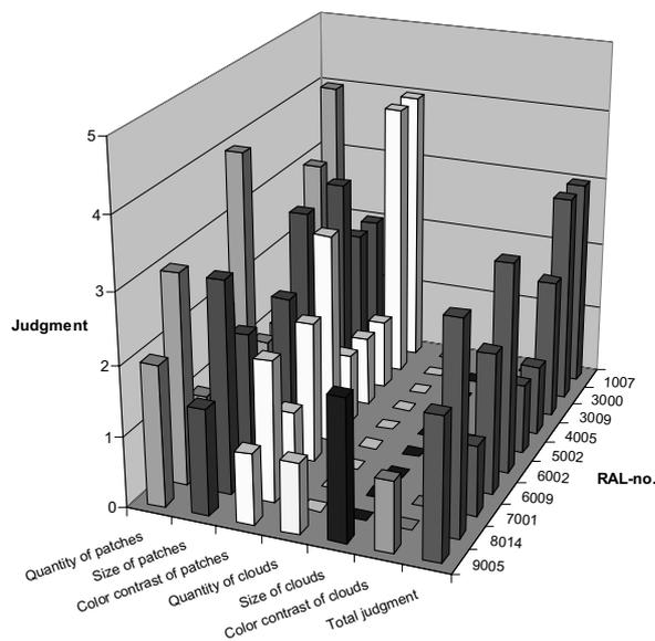
Figure 1. Results of visual judgment of 10 weathered paint samples after 5 years of weathering.
