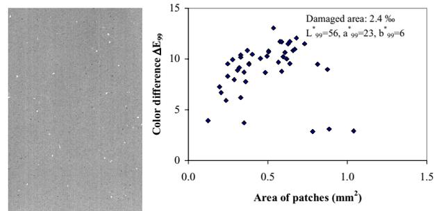
Figure 2. The left panel shows an image of patches on a weathered paint sample (RAL 3000) after 5 years of weathering. The right panel shows color differences between patches and homogeneous background versus size of patches of that sample. 2.4 % of measured area are damaged by patches.
