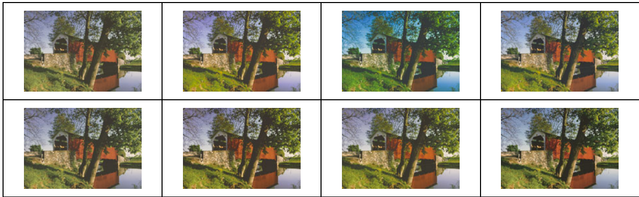
Figure 2. An sRGB image processed through different workflows for the HP DesignJet 10ps inkjet printer with semi-glossy proofing paper (top row) and the HP-Indigo 3000 LEP printer with glossy paper (bottom row). Left to right: offset CMYK data rendered as SWOP Relative Colorimetric, re-rendered (see text), native (no color correction), and RGB data printed with Perceptual rendering intent. The re-rendered hues are consistent with offset (SWOP). Color saturation is selectively expanded, and closer to direct RGB rendering. The amount of expansion (or compression) depends on the native color gamut of the digital printer being used. Hue differences are especially noticeable in the native case.
