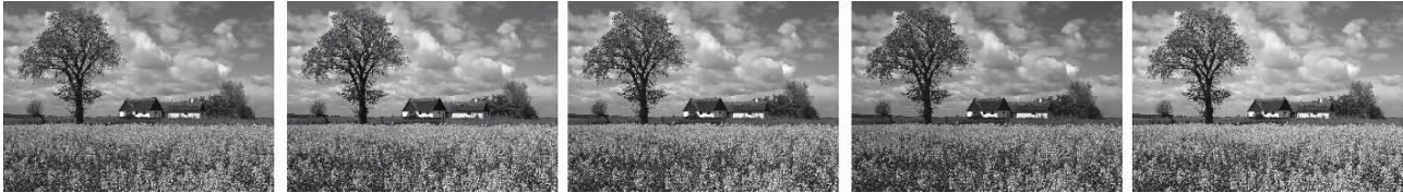
Figure 6. Cross-rendering a CMYK grayscale image separated for five CMYK spaces using re-rendering and GAT (see text). From left to right: separation profiles EuroScale, Gracol, SWOP, Toyo, and US Sheetfed Coated.
