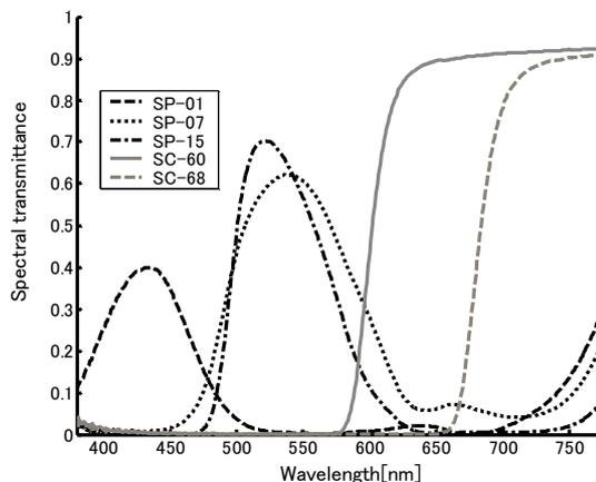
Figure 4. Spectral Transmittance of the filter
