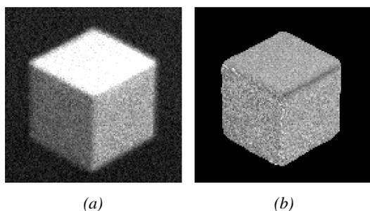
Figure 7. Shadow removal of box (a) spectral radiance image (b) spectral reflectance image
