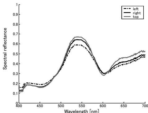
Figure 8. Spectral reflectance of three faces of the box
