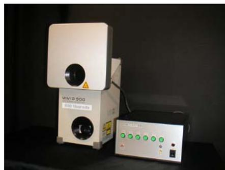
Figure 3. Modified VIVID 910 with multi-band filter unit
