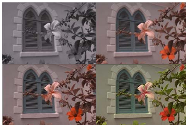
Figure 3. Partial reconstruction of the image. (a) Using only the first principal component (CPSNR=19.7) (b) Using 1 st and 2 nd (CPSNR = 21.6) (c) Using four (CPSNR =24.4) (d) Using five principal components (CPSNR =27.9).
