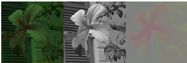
Figure 4. (a) Mosaiced color image according to the Bayer CFA, decomposed as (b) luminance plus (c) sub-sampled opponent chromatic channels.
