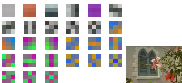
Figure 2. (a) Image (b) Spatio-chromatic representations of eigenvectors of the covariance matrix (with V = 3 ). Vectors are arranged in rows of decreasing eigenvalue magnitude.
