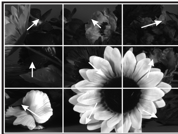
Figure 4: Translation vectors are determined for a set of subregions. Orientation and length vary throughout the image.
