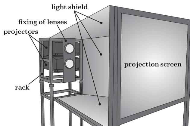
Figure 1: Experimental setup of a 6-primary display using two LCD-projectors. The spectral power distribution measured in the center of the screen is shown in fig. 2.
