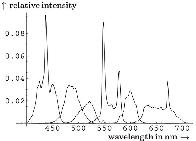
Figure 2: Spectral power distribution of the laboratory model (measured in the center of the screen).
