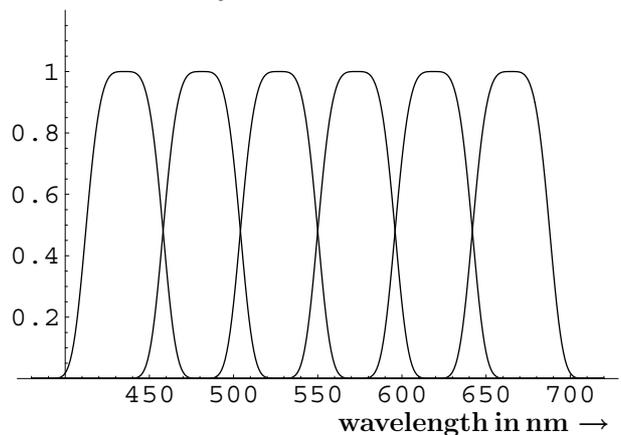
Figure 6: Spectral power distribution of six ideal primary channels with smooth spectral aperture functions.
