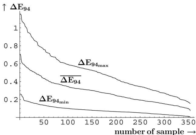
Figure 7: Color differences in CIE  $\Delta E_{94}$  between original color stimuli of the *Vrhel* data set and simulated reproduction using the spectral power distribution of the laboratory model (see fig. 2), calculated for 24 observers (see fig. 4) with illuminant  $D_{65}$  (ordered by size).
