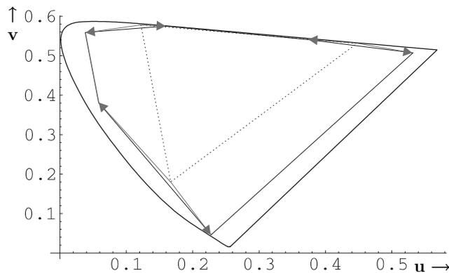
Figure 3: Color gamut of the 6-primary display given in the CIE 1976  $u'v'$ -diagram. The arrows are marking the split of the primaries of the projectors by additional filters. The triangle represents the color gamut of the original projectors.
