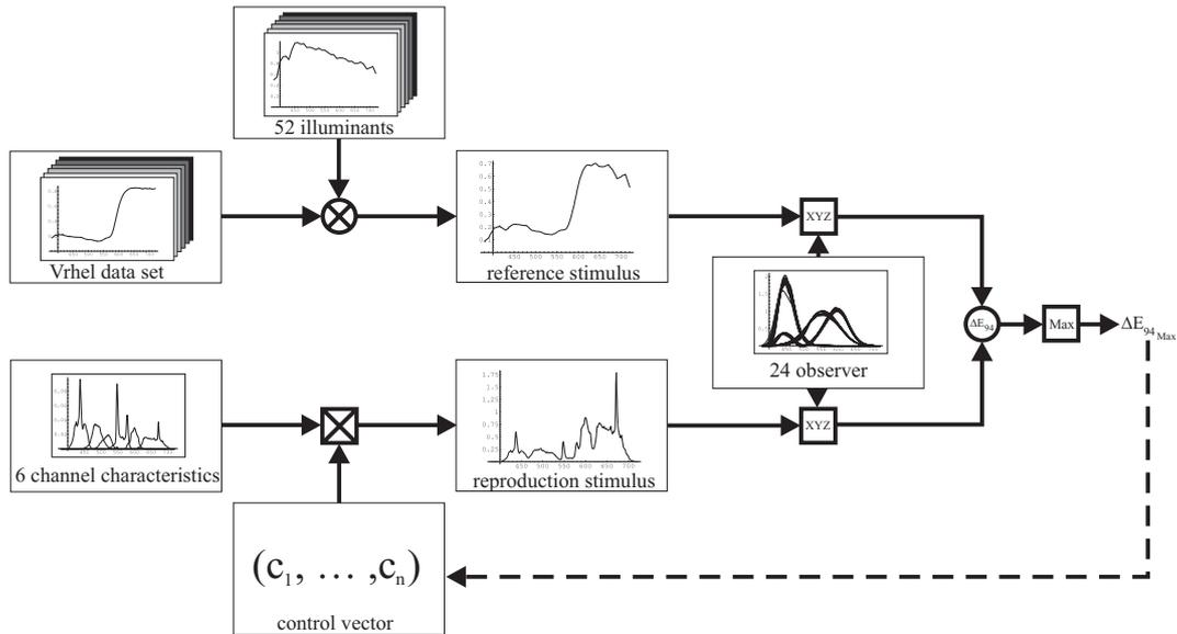
Figure 5: Simplified principle of the algorithm (without attention to the black offset, the change of the error criterion, and regards to parallel-serial processing)
