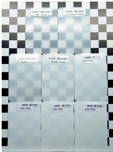
Figure 3. HDPE chips with different TiO<sub>2</sub> content
