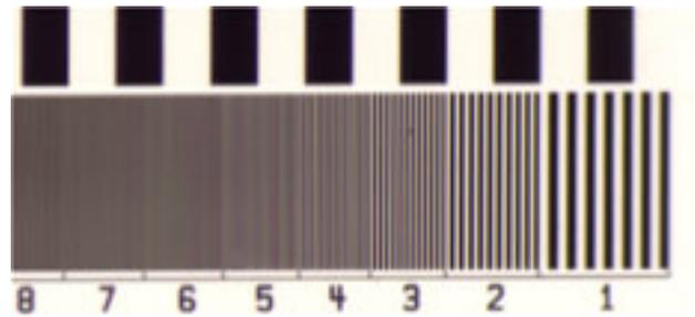
Figure 7. Image of the vertical test bars of the FBI SIQT test chart taken with a scanner speed of 1mm/sec, calculated using CIE 2° Observer and D65 illuminant. Numbers indicate the frequency regions in lp/mm.
