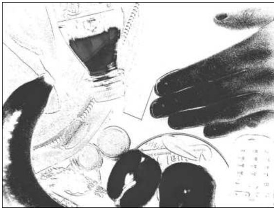
Figure 9: Thresholded ratio between two images captured with filters of \lambda=830\text{nm} and \lambda=950\text{nm} , respectively, centre wavelength.
