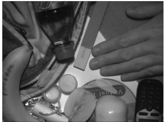
Figure 8: Image with human skin and other every day materials captured under tungsten light with a JAI CV-M4+ camera and an optical bandpass filter with \lambda=830nm centre wavelength and 20nm bandwidth.
