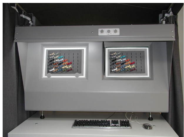
Figure 2: SpAIXview: Multispectral viewing workstation.
