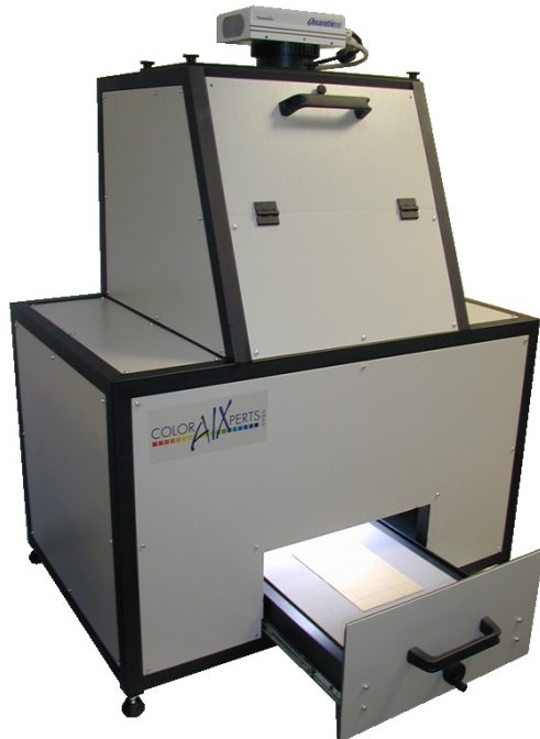
Figure 1: SpAIXscan: Multispectral scanning system.
