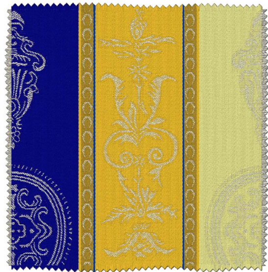
Figure 4: Sample fabric simulation of a weaving CAD software (Jacquard type).
