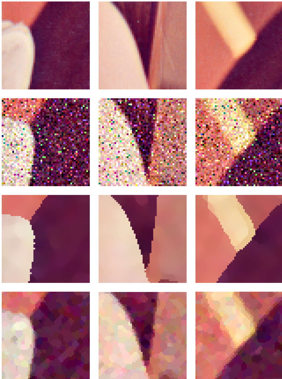
Figure 2. Comparison of the new algorithms with the standard vector median. From top to bottom : parts of the Lena test image from Fig. 1, images distorted by 4% impulse and Gaussian noise \sigma = 30 , images filtered with the new algorithm and the results obtained with the vector median.
