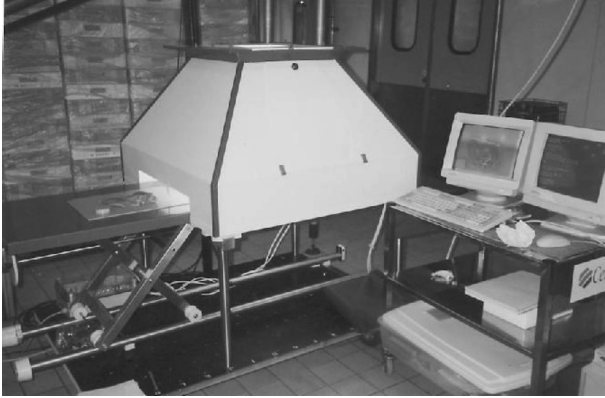
Figure 1. Color vision system for study of turkey breasts
