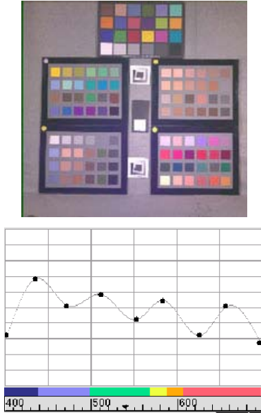
Figure 7: Example of watermark signal embedded to the spectral distribution of the viewing illuminant I_{\tau,\beta,\alpha}(\lambda) = I_{\alpha}(\lambda) \pm 10\% I_{\alpha}(\lambda) with \alpha = 1 .
