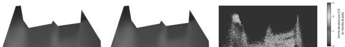
Figure 6. From left to right: original anisotropic floor, floor simulated as an isotropic object, and the error image between the original and the rerendered images.
