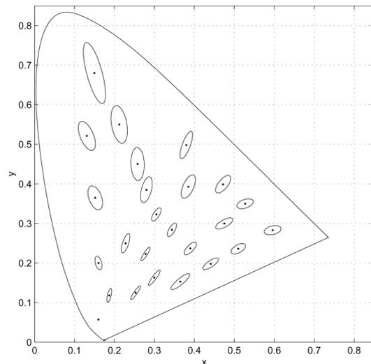
Figure 1. The MacAdam ellipses. The axes of plotted ellipses are 10 times their actual lengths.<sup>5</sup>
