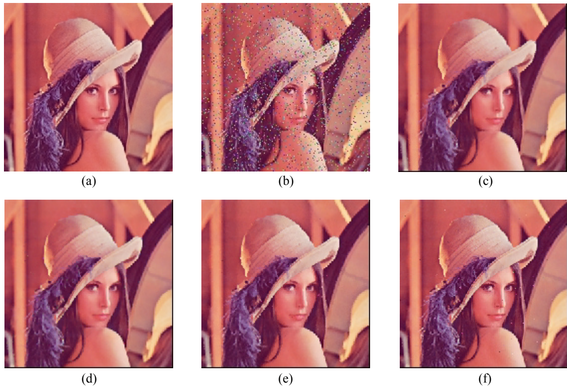
Figure 2. Achieved results (a) Original image (b) 10% impulse noise (c) Output of vector median (d) Output of marginal median (e) Output of BVDF (f) Output of proposed Method
