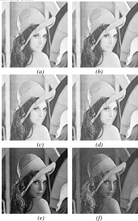
Figure 4. a) Watermarked Red channel of the image using the second LSB, b) Watermarked Red channel with a compression at 100% of quality, c) at 80% of quality, d) at 60% of quality, e) Watermarked Green channel with a compression at 80% of quality, f) Watermarked Blue channel with a compression at 80% of quality.
