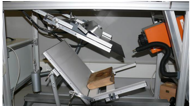
Figure 4. Set-up for IR-watermark detection with a book cradle that can be adapted to sensitive books and with the heated copper plate in its highest position for choosing the page under investigation. The camera (orange) is focused on the plane were finally the paper under investigation will be.
