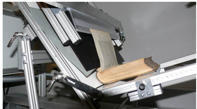
Figure 5: Detail of the setup showing that every single leaf of the book will be held flat in a certain position by a vacuum bar.
