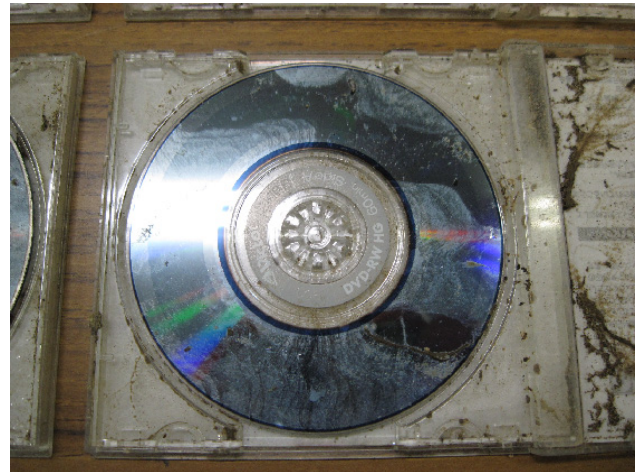
Figure 10 : Optical disc soiled with seawater and mud.
