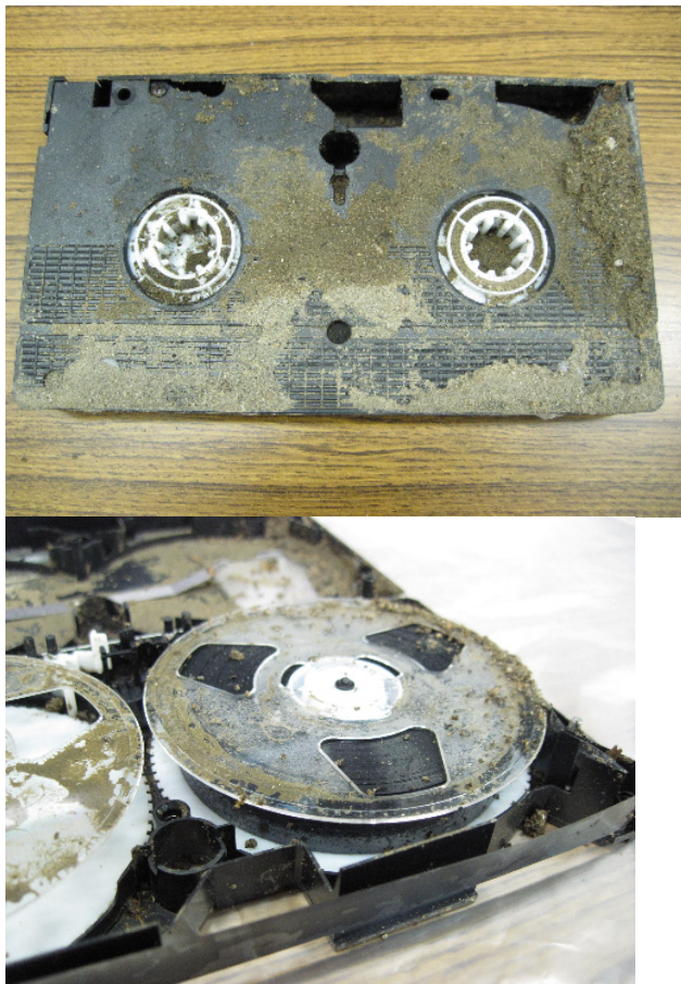
Figure 11 : Magnetic tape soiled with seawater and mud
