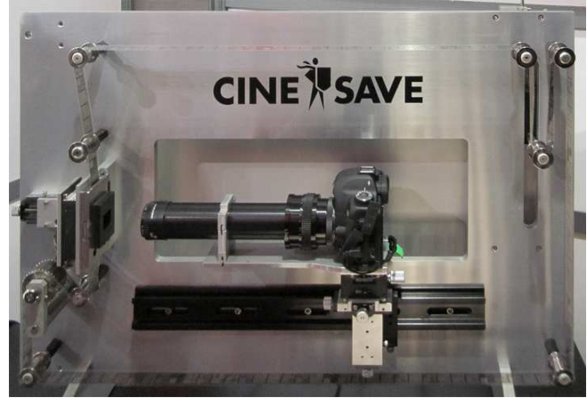
Figure 4. The film scanning setup constructed in the CineSave project.
