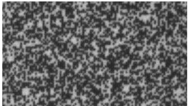
Figure 7. Data points exposed on Fuji Eterna RDS film using the Arche laser recorder (grid space: d = 6 \mu\text{m} ).
