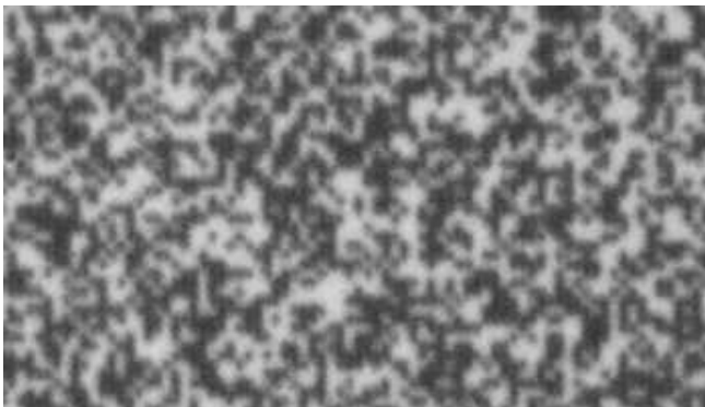
Figure 6. Data points exposed on Fuji Eterna RDS film using the ARRILASER (grid space: d = 7.57 \mu\text{m} , diagonal grid).
