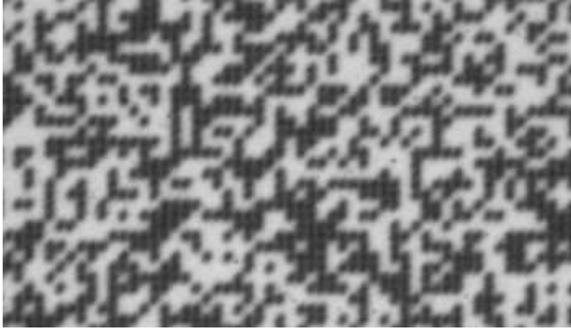
Figure 3. Data points exposed on Fuji Eterna RDS film using the ARRILASER (grid space: d = 10.71 \mu\text{m} ).
