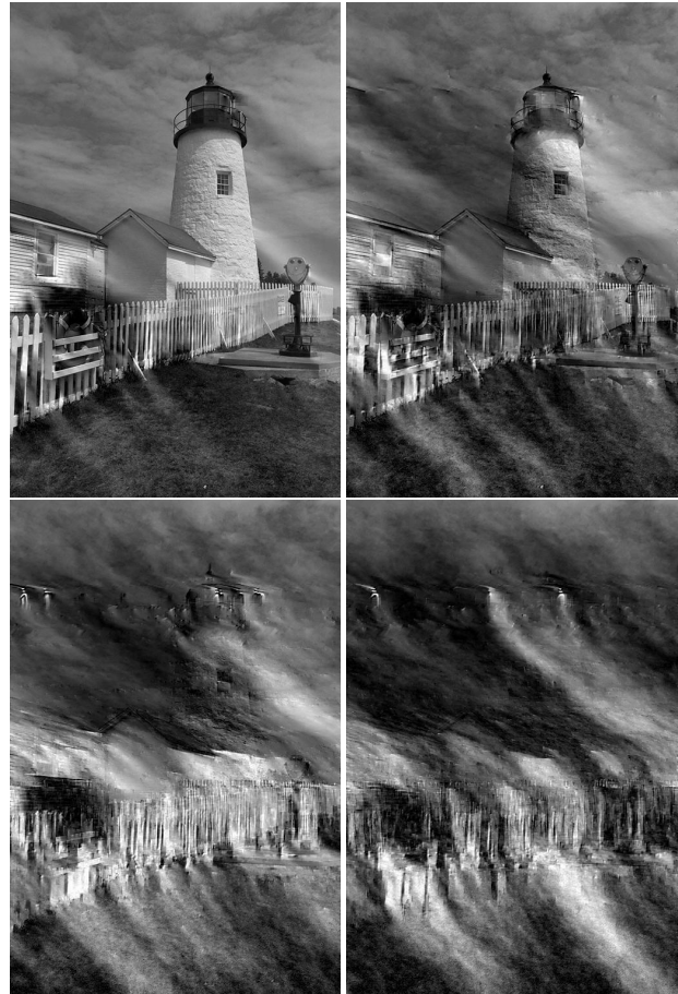
Figure 10. Even heavier error rates including bursts are applied to this second set of pictures. The image file stay always readable. Size is 512 \times 768 pixel = 3145728 bits (8 bits/pixel luminance channel). From left to right, top to bottom : 0.01% corruption (314 bits altered), 0.1% (3145 bits), 1% (31457 bits) and 10% (314572 bits - that means that 1 bit out of 10 is swapped)
