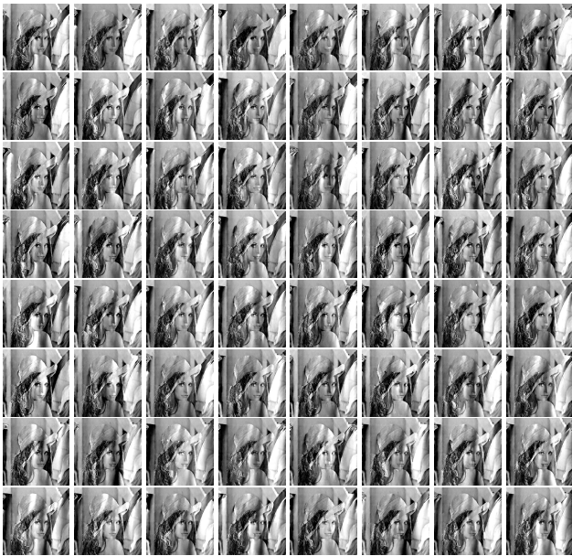
Figure 9. Storage using our compression scheme. Corruption of 1000 random bits per file (10x more than the JPEG2000 ones). By applying only 100 random bit errors to each file, the EDC/ECC recovers all the data. The average compression ratio is 0.55 (better than JPEG2000).
