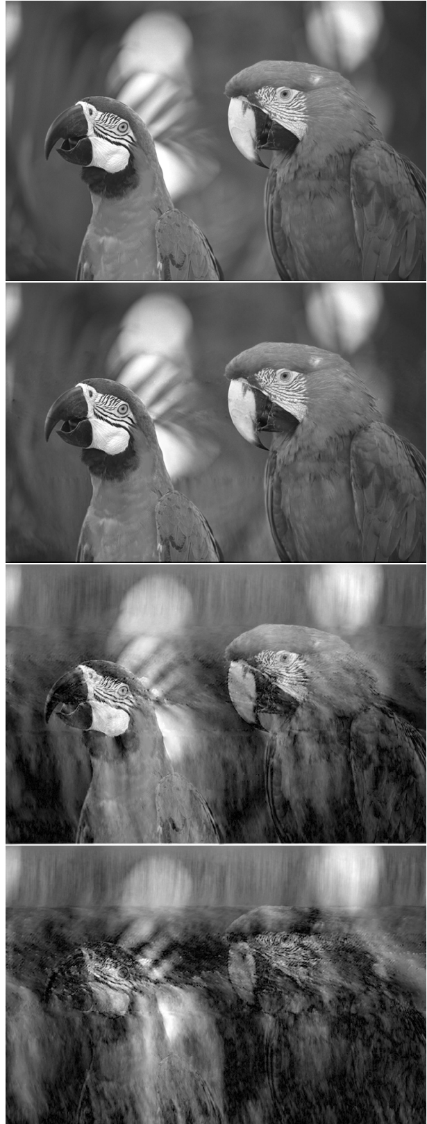
Figure 12. Size is 768 \times 512 pixel = 3145728 bits (8 bits/pixel luminance channel). From top to bottom : Original, 0.01% corruption (314 bits altered), 0.1% (3145 bits) and 1% (31457 bits)
