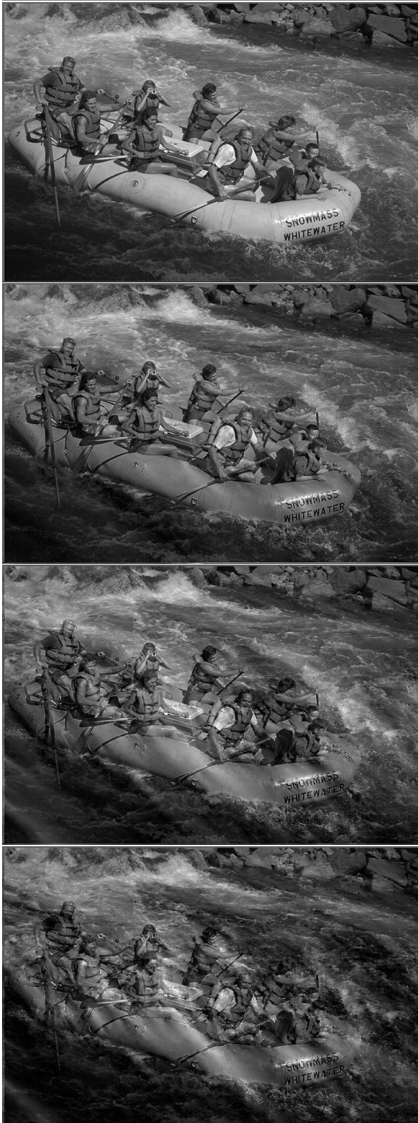
Figure 11. This set of pictures illustrate the behaviour of the compression algorithm if the amount of bit errors exceed the ECC capacity. Size is 768 \times 512 pixel = 3145728 bits (8 bits/pixel luminance channel). From top to bottom : Original, 0.01% corruption (314 bits altered), 0.04% (1258 bits) and 0.07% (2202 bits)
