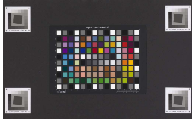
doing so we've come up with just one test chart instead of the usual four (Color, Sharpness, Uniformity and distortion).
