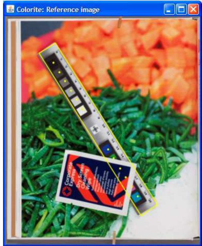
Illustration 2. The SURF image matching algorithm often manages to locate the target even in cluttered images and under partial occlusion. Compared to Illustration 1, the image matching accuracy is slightly reduced.
