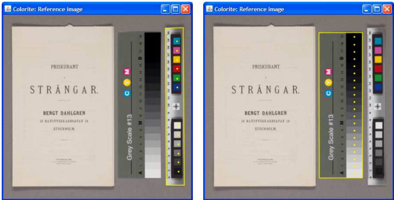
Illustration 1. Different targets in the reference image are located by changing the target image. The target in the left image is custom made at the Division of Digital Production and based on the X-rite ColorChecker Mini. The target in the right image is the common Kodak Q-13. The images appear to be too dark because the viewer does not support color management.
