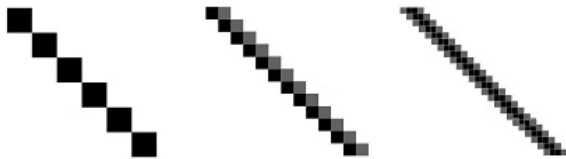
Figure 3. Absolute sample frequency: one pixel or line represents one image detail; minimum sample frequency: two pixels or lines represent one image detail; practical sample frequency: four pixels or lines represent one image detail.
