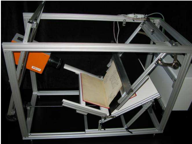
Figure 14. Set-up for detecting watermarks in books. The photograph shows the infrared set-up used in the examination of a historic book.
