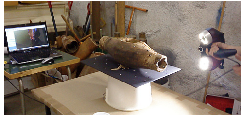
Figure 6. Optical hand-held scanner which produces the 3D model mesh with texture instantly (E. Hannus/Viva3)
