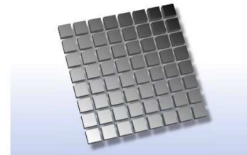
Figure 1. An area array—each photosensor contributes one pixel to the image. © 2004 Adobe Systems Incorporated. All rights reserved.
