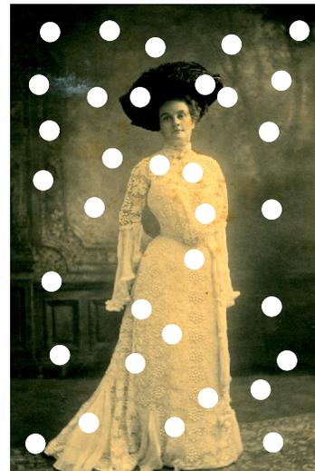
Figure 3: Example print with measurement locations indicated
