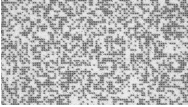
Figure 1. Microscopical image of exposure points ( P = 2 amplitude levels, d = 9 \mu\text{m} grid space).
