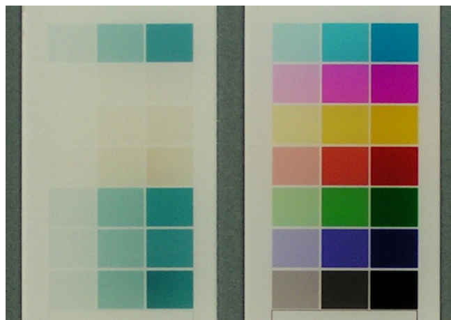
Figure 6 “Enclosure / Picture Frame Effect” caused by strong yellow dye fading in face-mounted colour photographs on white-pigmented polyester
