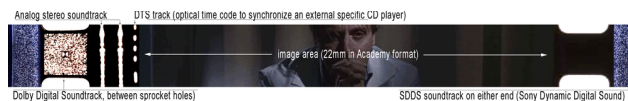
Figure 1. 35mm film strip showing modern digital soundtracks along the analog VA soundtrack.
