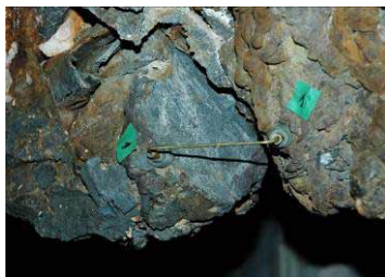
Figure 2. Fissure Formation in WTC Steel Composite
