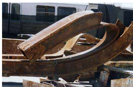
Figure 3. Distorted WTC Steel Beam
