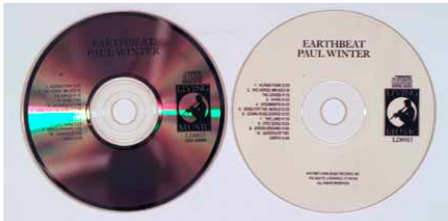
Figure 7: Discs 69C and 69D after 500 hours accelerated aging
