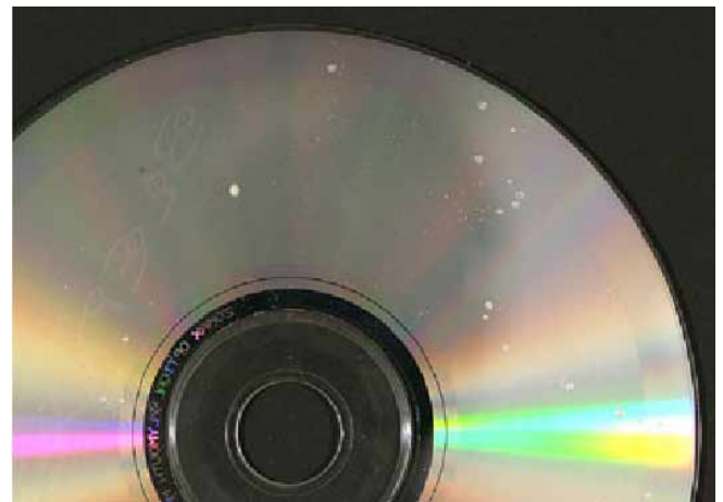
Figure 6: Spots on CD representing degradation of polycarbonate
