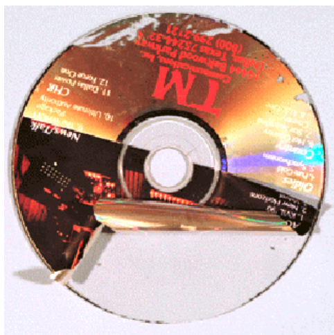
Figure 3: Delamination of the reflector after thermal cycling
