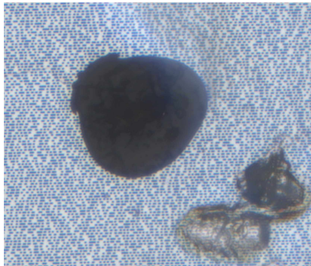
Figure 2: Photomicrograph of a 'pin-hole' defect in the reflector among data pits
