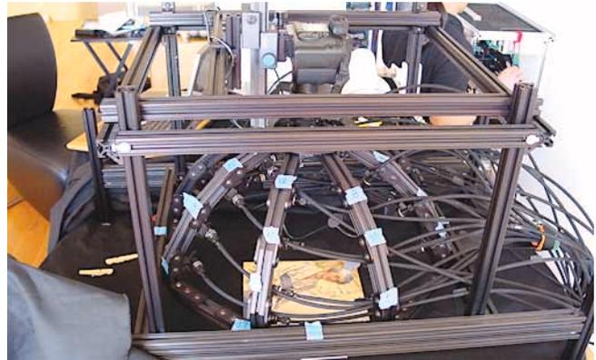
Figure 1. Reflection Transformation Imaging apparatus modified for spectral imaging
