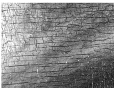
Figure 22: Horizontal cracks (veil).
