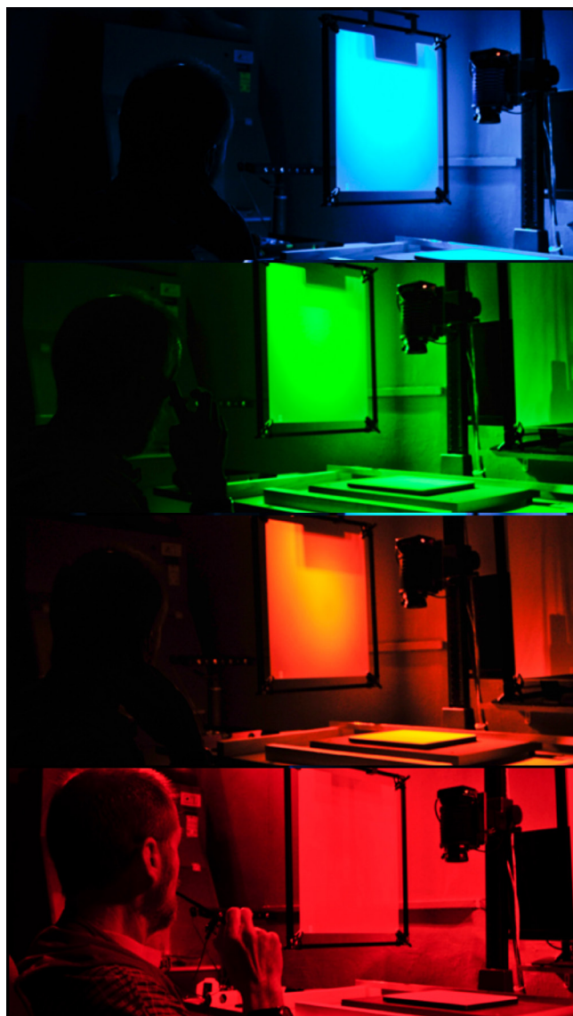
Figure 1. A composite of four photographs showing Ken Boydston at the new Israel Museum facility in Jerusalem that was established in 2011 to image and monitor the Dead Sea Scrolls. The photographs show four of the twelve narrow-band wavelengths of the LED illumination employed with the multispectral imaging system. (Photographs and digital composite by Shai Halevei)
