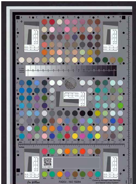
Figure 3: FADGI ISO 19264 test target
