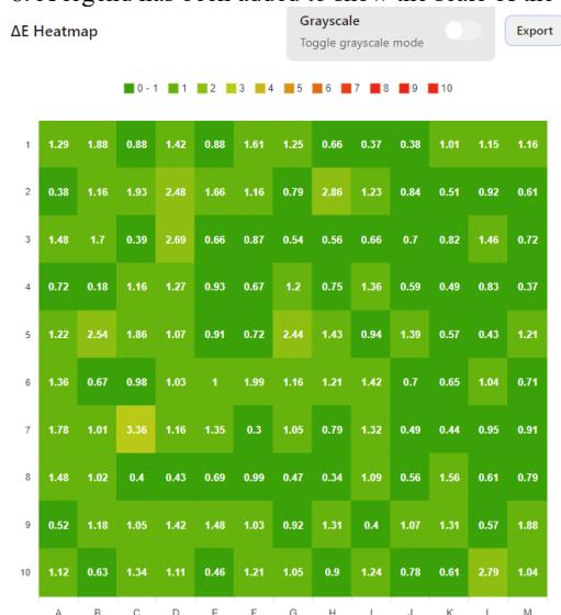
Figure 8. Screenshot of the color difference heatmap in Beyond RGB 2.5. Each square represents one patch in the calibration target.
