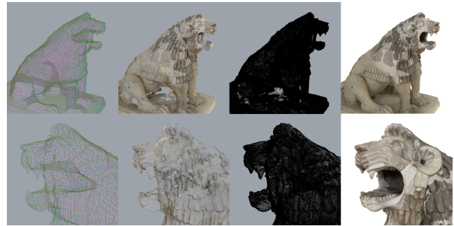
Figure 1. The same heritage model in four representations - from left to right: our variable-axes topographic lines, a point cloud, a wireframe, and a mesh. The top row shows the full model; the bottom row shows a zoomed-in detail.
