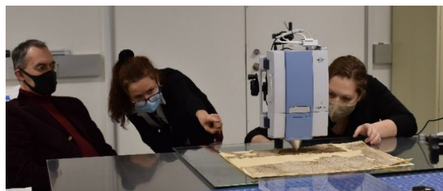
Figure 2. Colleagues and PRTD Heritage Scientists working on Magna Carta Documents with Fourier Transform Infrared (FTIR) Spectroscopy.
