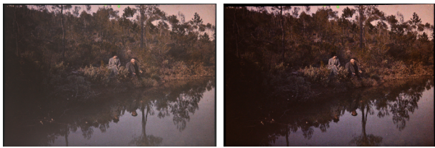
Figure 5. The difference between not covering the lightbox surface around the autochrome plate (left) and covering it with a fully-absorbing black sheet (right) is obvious with the naked eye in terms of image contrast.
