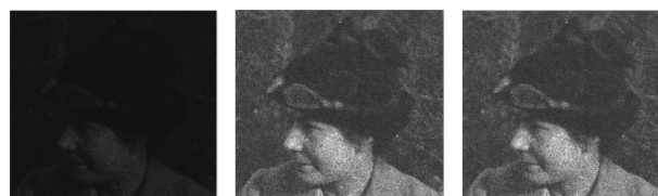
Figure 3. Zoomed-in section of the autochrome. Left: Image exposed for the backlight (exposure time: 25 ms). Middle: Exposure-compensated image (exposure time: 25 ms). Right: Image exposed for the autochrome (exposure time: 300 ms.)
