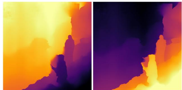
Figure 6. Disparity maps of correctly transposed stereo pairs: left view with positive values (left) and right view with negative values (right), enabling automatic detection of pseudoscapy.
