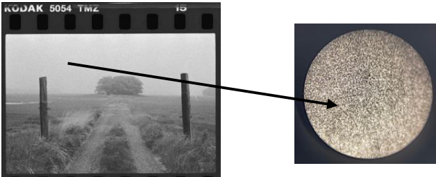
Figure 4a: 35mm black and white film grain measurement (TMAX) 5.3 microns; imaged at 4800 ppi.
