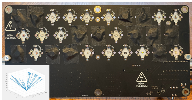
Figure 2. Standard MISHA light panel modified to allow single LED illumination. The inset shows the 22 light direction vectors estimated from images of a mirrored ball.
