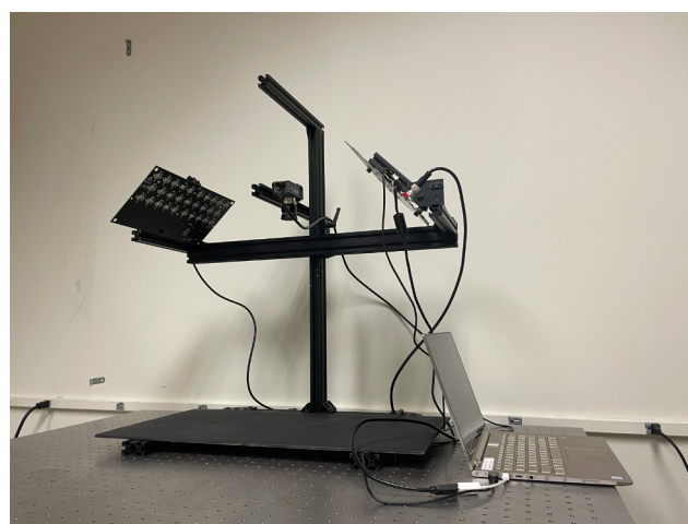
Figure 1. The MISHA multispectral imaging system.
