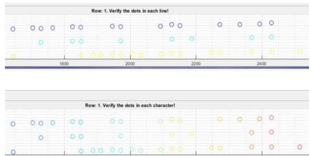
Figure 7. Each dot in a line of characters should be correctly grouped into one of the Braille rows (top, middle, or bottom), and one of the characters in the line.
