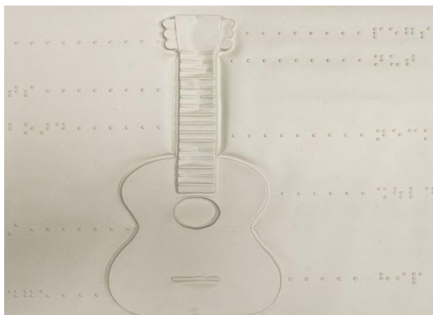
Figure 9. The paper sample with an embossed guitar shape
