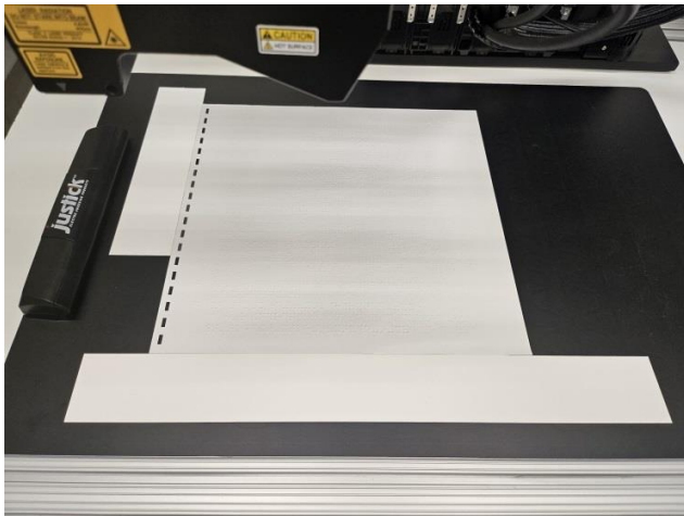
Figure 5. Alignment of the braille paper along the scanning direction
